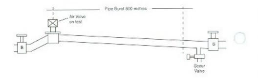
In an actual test on a gravity pipeline, the pipeline burst 800m away from the air valve on test, proving that the induced pressure, although attenuated by the pipeline structure was sufficient to damage the pipeline 800m away from the source of the pressure rise.
