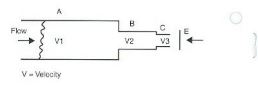
In the model A = the main pipeline and has an internal diameter of 356.82 mm = 100 L/meter. B (riser) = 112.83 mm = 10 L/meter. C = air valve which has an outlet of 100mm Dia.
